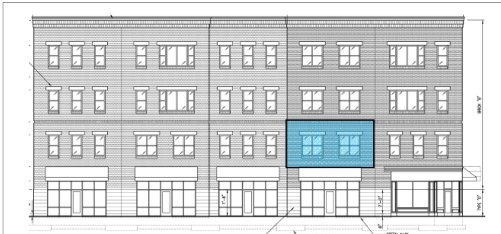
Figure 33– Panel #5, Erection Sequence-4; Located Along 3 rd Street
